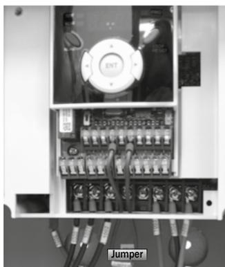
Figura 6A - bornes com jumper
