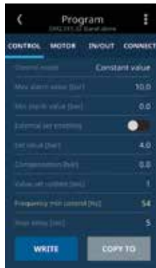
Figura 19 - Tela Valor Frequency min control alterado
